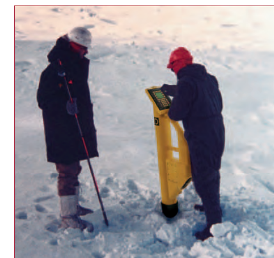
Fig. 2. The C-Scan detector unit at work on the bed of a 10-m deep frozen river in Canada.
